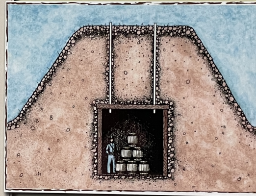
Cross-section of the powder magazine.
