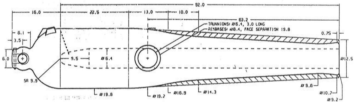
32-pounder Bureau of Ordnance Gun of 4,500 pounds, Preponderance, 350 pounds; weight ratio, 141 with round shot; bore length 14.4 calibers. The hatched area designates the specified rough casting. SOURCES: RG74 E202, red series drawings 972 & 1034; black series drawing 3171.
