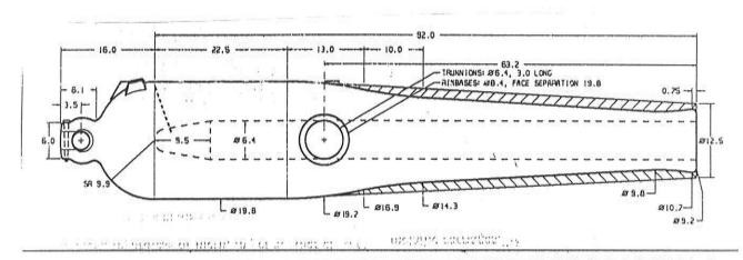
32-pounder Bureau of Ordnance Gun of 4,500 pounds. Preponderance, 350 pounds; weight ratio, 141 with round shot; bore length 14.4 calibers. The hatched area designates the specified rough casting. Sources: RG74 E202, red series drawings 972 & 1034; black series drawing 3171.
