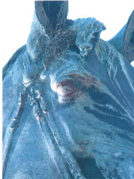
Fig. 6. View of the proper right side of the head of the horse. Please note the streaking, and contrast between the green and black corrosion which is disturbing the design of the sculpture. Please also note large brown areas. It appears that these spots were recently abraded to bare metal either by incorrect graffiti removal, or someone climbing the sculpture.
