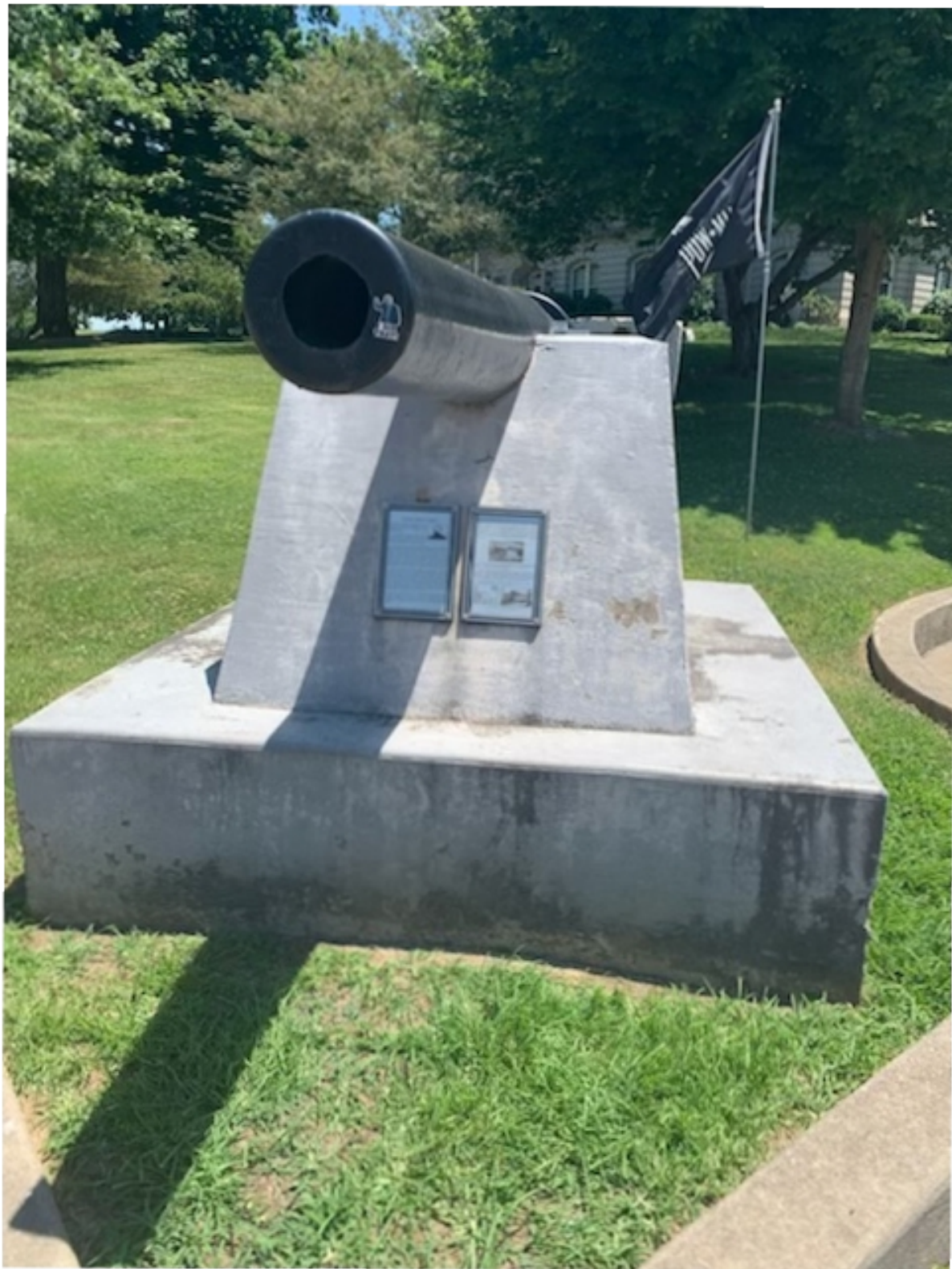
4.2 Army Parrott Rifle, Iron, 5 RH rifling, WPF Foundry Registration #209 , no inspector initials , FDY# 753, Made 1863, Weight 4175
